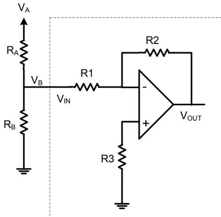
Fig. 2. Loading effect of the inverting amplifier
