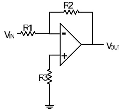
Fig. 1. Inverting amplifier
